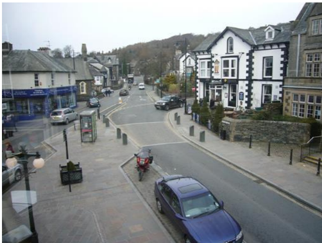
Windermere High Street - Pedestrian crossings with change of surface material, cycle parking options, and sensitively designed bollards.
