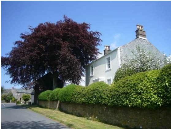
Fig. 26 A large copper beech beside Greenbank, a mid-19 th century dwelling with unusual slate-hanging on the gable end.
