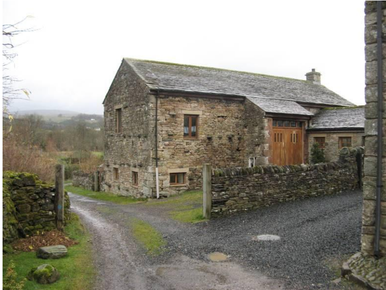
Fig. 13: The Barn is one of a number of former agricultural buildings that have been converted to residential use. The former cart entrance is clearly visible and the structural 'throughstones' are a distinctive feature.
