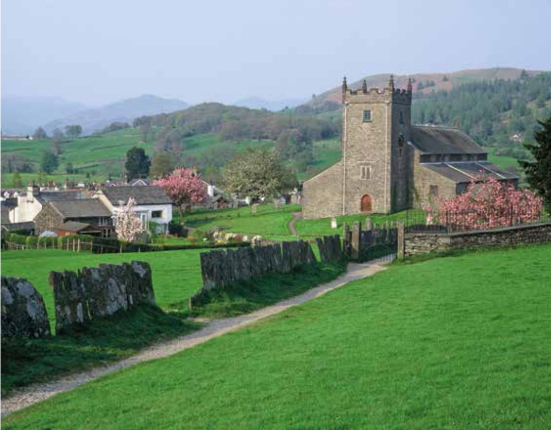
FIGURE 3.5 View of Hawkshead and the church of St Michael and All Saints. The view includes a fine example of a shard fence constructed from interlocking vertical slates.
