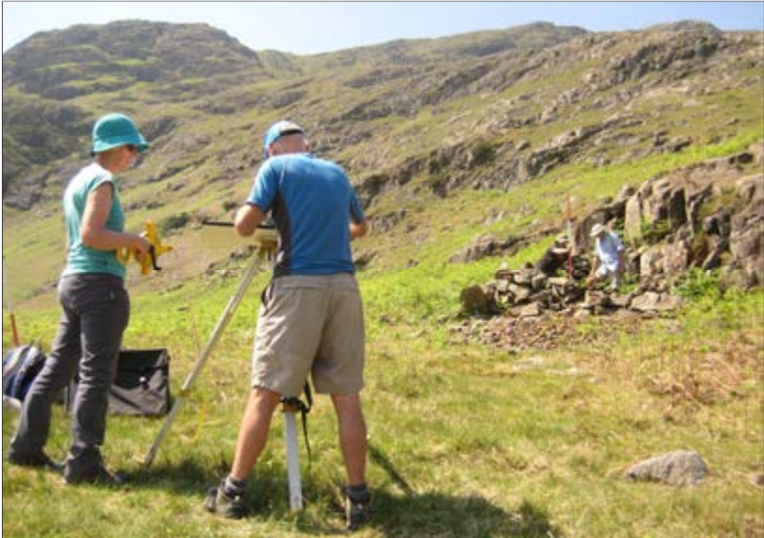
Plate 3: plane table survey underway at Tilberthwaite mine.
