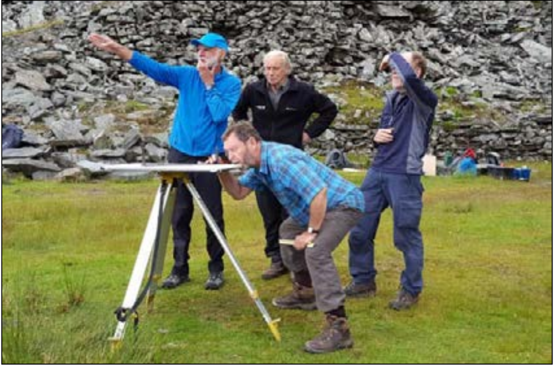
Plate 2: plane table survey under the watchful eye of John Pickin (adjusting alidade)
