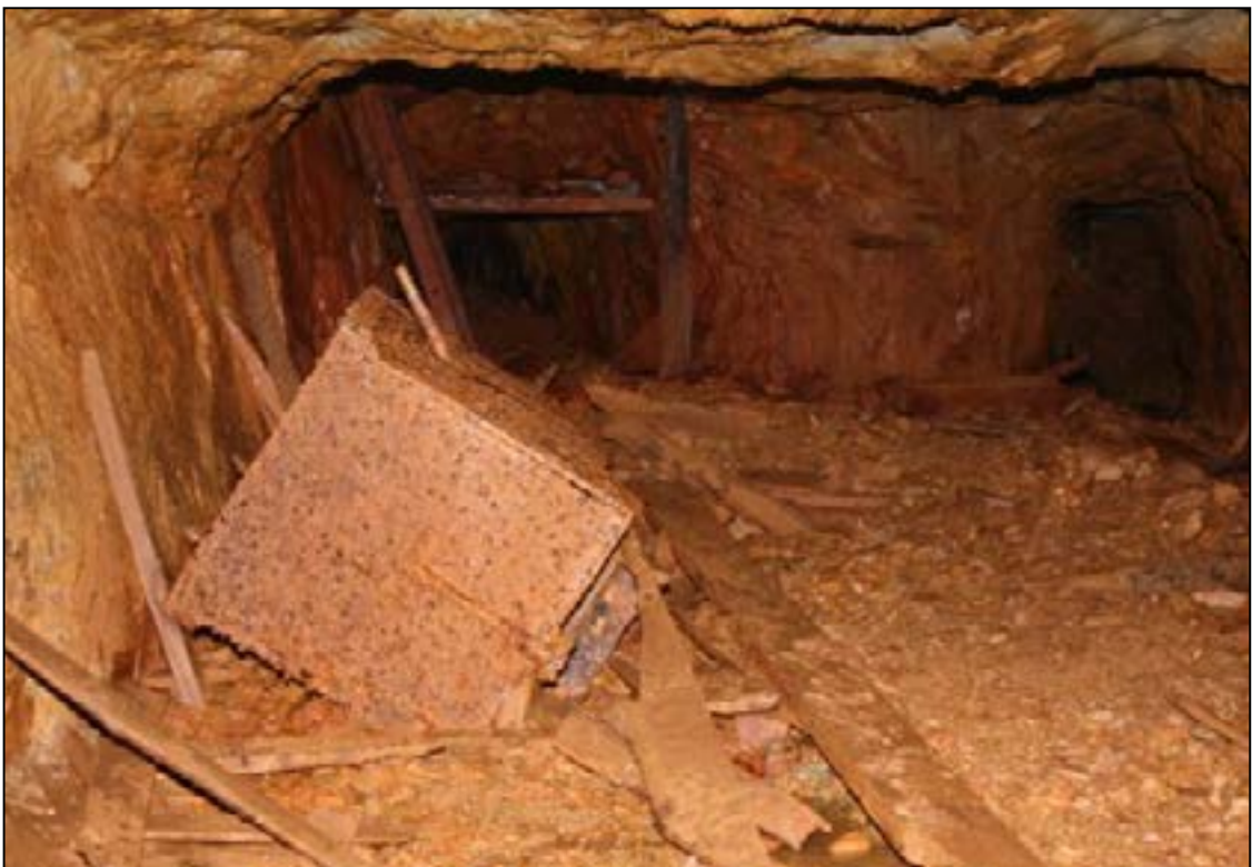
Plate 50: mine tub surviving in situ in the Horse Crag Level. Photograph courtesy of Warren Allison
