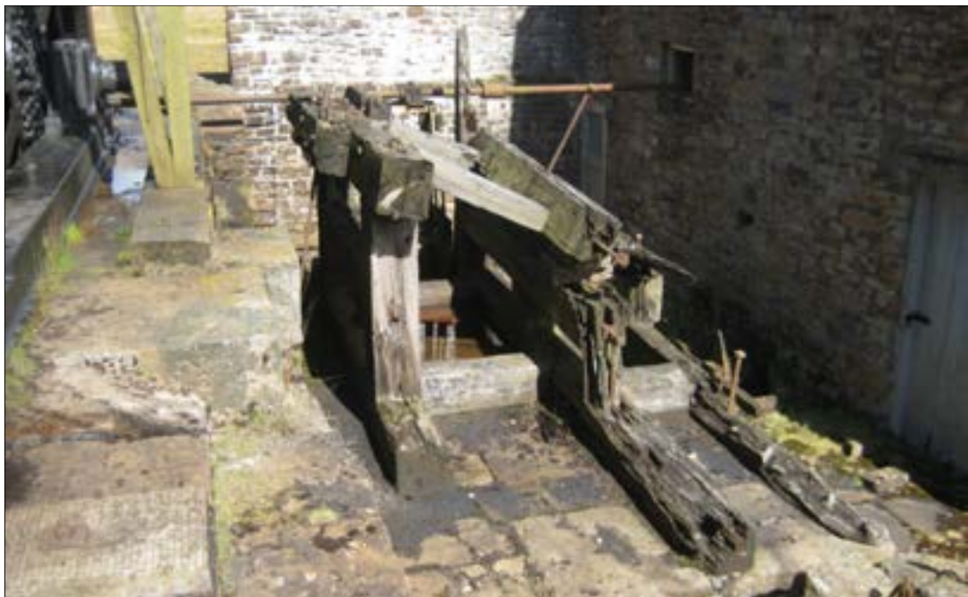
Plate 14: ore crusher supports at Killhope mine, Co. Durham.
