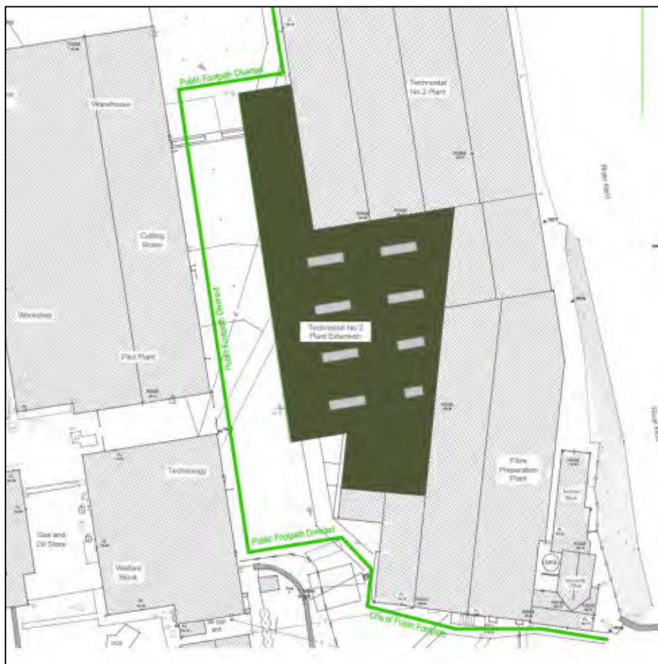
Planning application – extension is blocked in dark sage colour, and initial diversion proposal shown in light green
